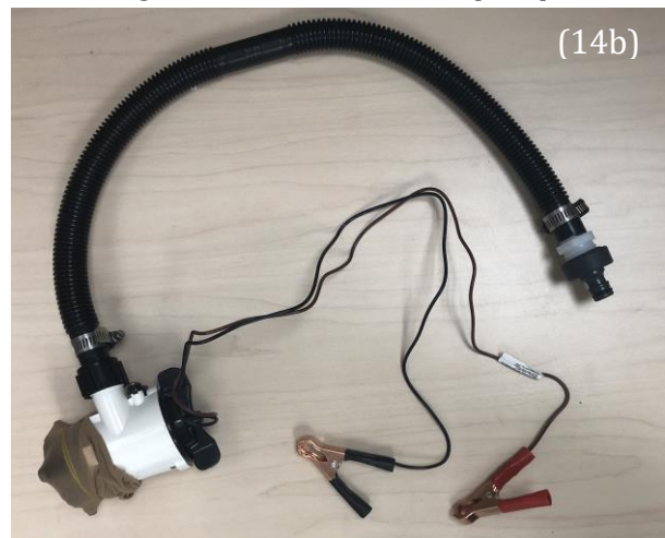
Figure 14. Bilge pump preparation: (14a) identifies the materials that will be required to prep the bilge pump and (14b) depicts how the bilge pump should look when put together.
