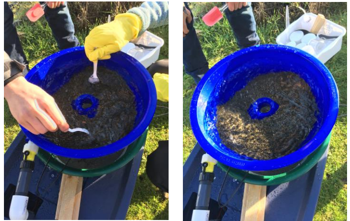
Figure 7. Depicting how to agitate the sediment in the blue bowl.
