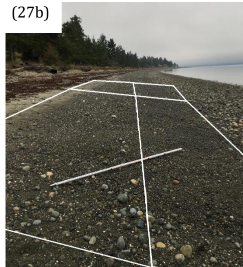
Figure 27. An example of how to visualize the sampling area to collect the representative sample: (27a) breaking the 30 m by 5 m into quadrats, and (27b) the quadrats drawn out on a beach.
