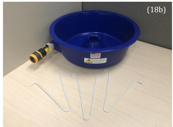
Figure 18. Blue bowl concentrator preparation: (18a) identifies the materials that will be required to prep the blue bowl and (18b) depicts how the blue bowl should look when put together.
