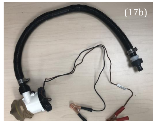
Figure 17. Bilge pump preparation: (17a) identifies the materials that will be required to prep the bilge pump and (17b) depicts how the bilge pump should look when put together.
